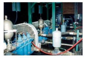
Pulsation and suction dampeners are used on pumps in many industries. Pictured here is a bank of pumps used for high pressure washing in a food processing facility
